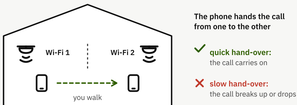
Figure 7. Moving between two Wi-Fi points. Inside a house with two Wi-Fi points, the phone hands the call from one to the other as you walk.
