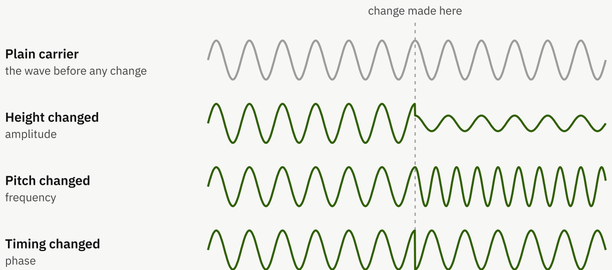
Figure 8. One wave, three ways to change it. Each wave starts the same. After the dashed line, one thing changes. The receiver watches for those changes and reads them as numbers.
